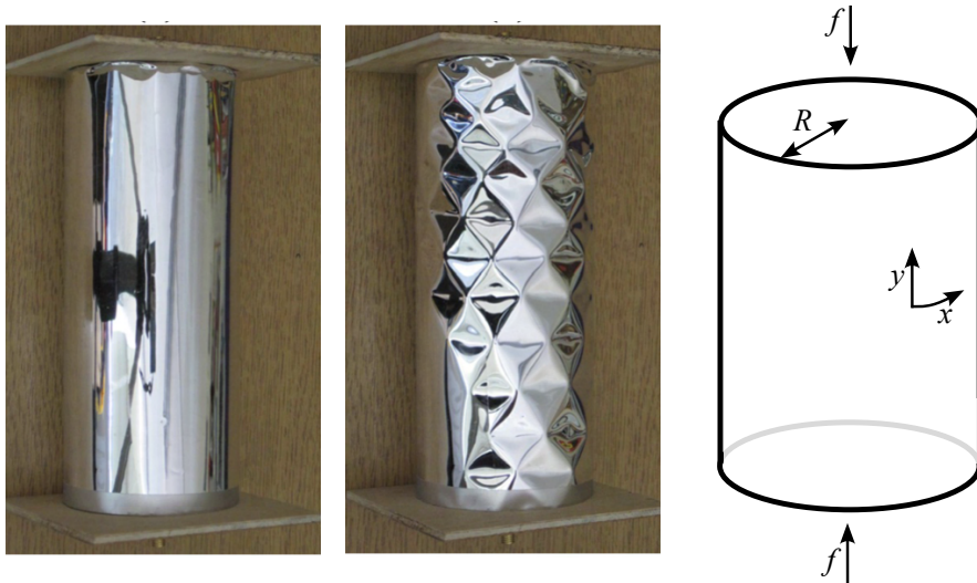
Figure 14: Left: A cylindrical shell, about to be squashed vertically (axially). Middle: The load force increases until a sudden instability occurs and the shell jumps to another shape. Usually the shape on the right would be seen only very briefly, en route to some less regular shape; here the nice pattern has been preserved with a trick (can you guess what’s inside the cylinder to achieve this?). This ‘Yoshimura’ pattern also comes up in origami theory! Photos from Seffen+Stott, 2014. Right: Sketch of the setup.
