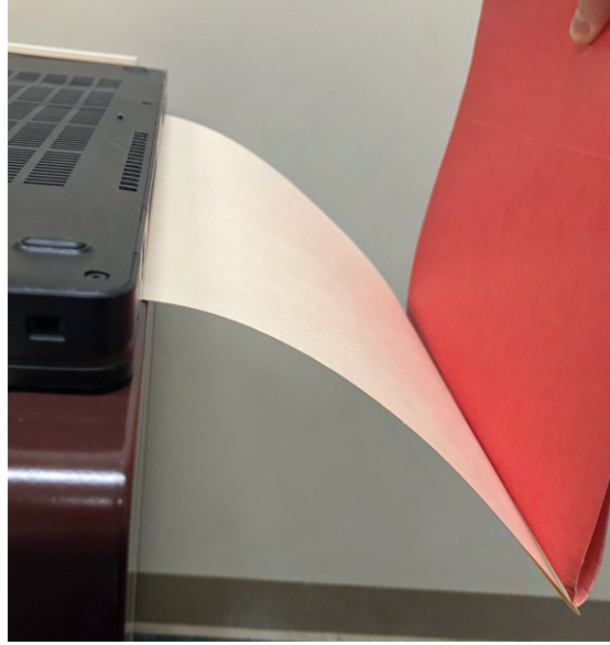
Figure 8: A plate cantilever (white) is ‘built in’ / clamped at its left-hand edge, and loaded at its right-hand edge by a load (red).
