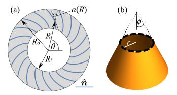
Figure 1. (a) An annular LCE sheet in the reference domain, with an axisymmetric spiral director pattern characterized by the angle  $\alpha(R)$ . (b) A truncated cone with semi-angle  $\phi$ . The dashed circle has curvature 1/r, and geodesic curvature  $k_g$  of magnitude  $\sin(\phi)/r$ .
