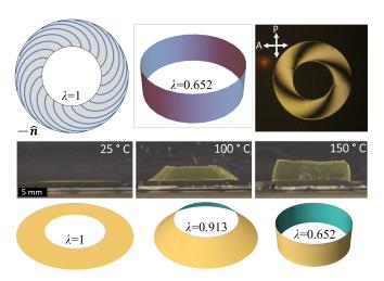
Figure 3. Director spiral (top-right) to morph an annulus into a cylinder (top-middle) at a design  $\lambda=0.652$ . Experiments (middle) and numerics (bottom) confirm the cylinder is attained, and also highlight the intermediate cone states en route.
